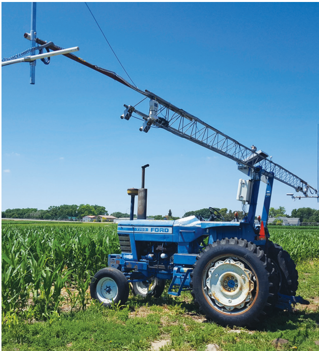
Figure 1. Mobile sensing platform at the University of Nebraska-Lincoln West Central Research and Extension Center (UNL-WCREC) in North Platte, Nebraska. Sensors include: four Apogee infrared radiometers (Apogee Instruments, Inc. Logan, Utah), two Holland Scientific crop circle sensors (Holland Scientific, Lincoln, Nebraska), two spectral reflectance sensors (Decagon Devices, Inc., Pullman, Washington), two GoPro cameras (GoPro, Inc., San Mateo, California), and one Apogee quantum sensor (Apogee Instruments, Inc., Logan Utah).
