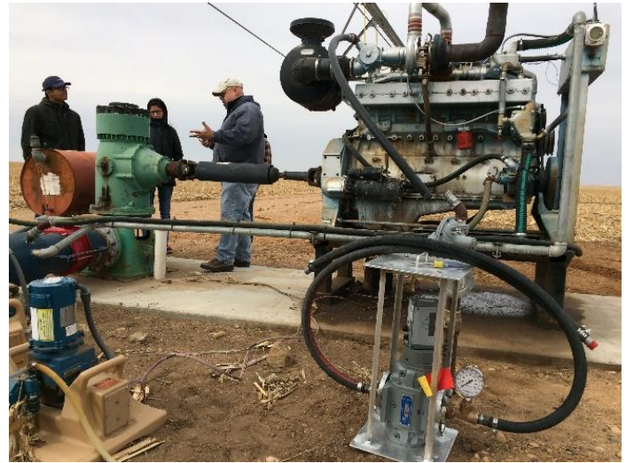
Figure 2. OSU's Mobile Irrigation Lab assesses producer's irrigation system water application and energy use efficiencies.
